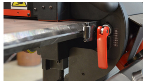
Convenient adjustment to plate thickness
